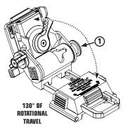
Push the flip release button (1) and position the Carriage in the stowed or operational position. Release the button to lock in place.
