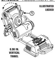
Placing the Lock Lever (1) in the unlocked position allows for vertical adjustment up and down. Turn the lever CW to lock.
