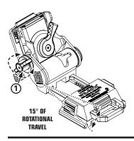
Turn the tilt angle adjustment knob (1) CW to raise the angle or CCW to lower the angle.
