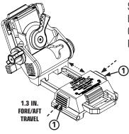
Simultaneously push both buttons (1) in to move the Carriage forward or backward. Release the buttons to lock.
