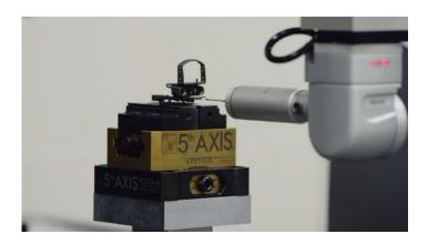
The tools used to conduct this "first piece" include the use of a coordinate measuring machine (CMM). These measurement tools are incredibly precise and are used to measure the parts to very tight tolerances with high accuracy. All of this is done to ensure the parts meet the drawings that were created by Wilcox and approved by the customer.
