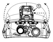
Step 1.) Depress the NVG Flip Button (1) and flip up to stow or down to deploy.
