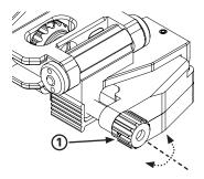
Turn the PD Adjustment Knob (1) until the proper position is obtained.
