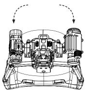
BINOCULAR BRIDGE PROVIDES 90° OF FLIP ANGLE FOR STOW **Step 2.)** Pivot the NVGs outward to stow flush against the helmet when not in use.
